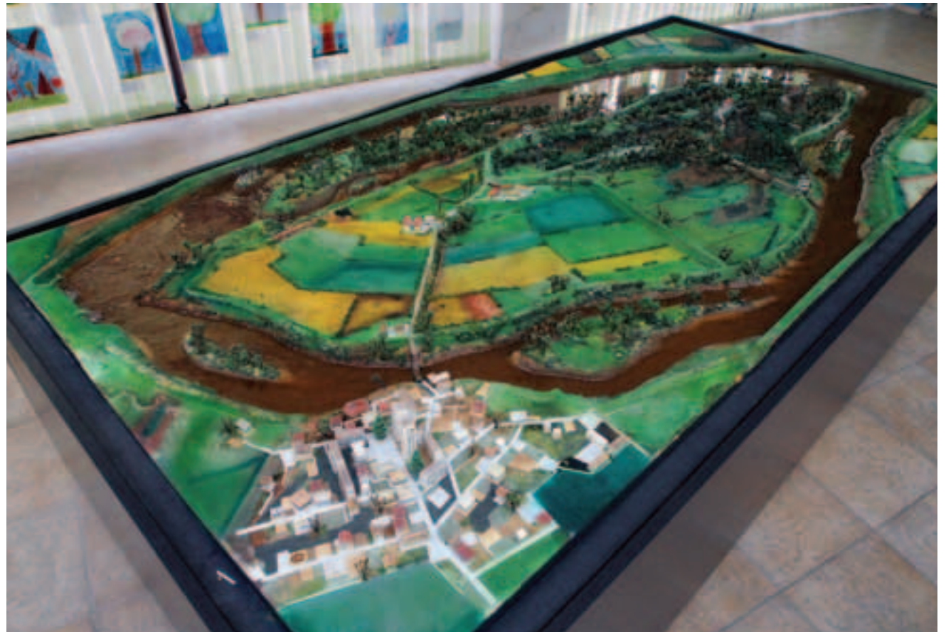
The 3D model of the Persin island in the Visitors Centre. It is possible to fill its channels with water by opening tiny valves and to observe an impact that flood makes on the island
