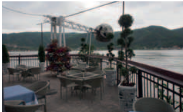
Before the Djerdap dam was built, navigation through the gorge was tricky and dangerous. Devices like this were used to show to boats priority of the pass in very narrow parts. Up: go. Down: stop and wait.
